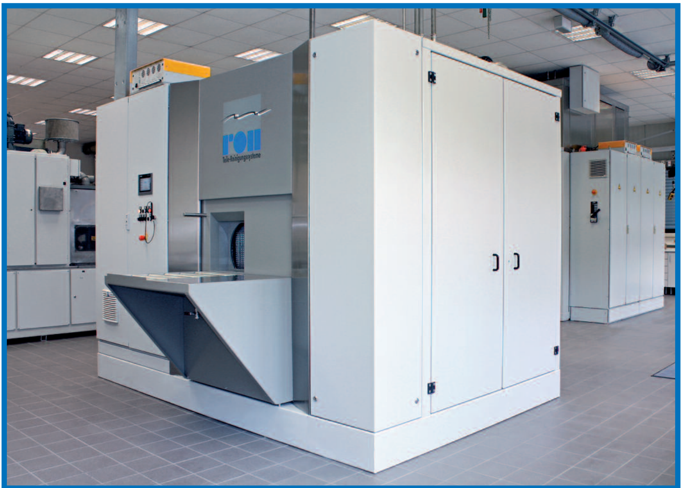
Single chamber flooding cleaning facility
