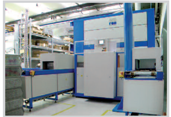
Single chamber facility with automatic charging and discharging device
